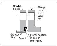
**Note:** Design of the Gruvlok Flange provides sealing only withthe special Gruvlok Flange gasket. Only Gruvlok Flange gaskets may be used with Fig. 7012 Gruvlok Flanges. 2.6 Align the Gruvlok Flange bolt holes with the mating flange bolt holes. Insert a standard bolt or stud through the bolt hole, and thread a nut on hand tight. Insert the next bolt or stud opposite the first and again thread the nut on hand tight. Continue
